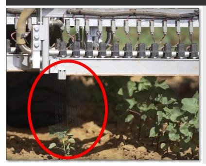
**Targeted spraying** mechanisms from OEMs and startups are beginning to enter the marketplace. Early estimates show that initial savings from herbicide application can be up to 90% **per pass**. Yet, questions remain as to the long-term effectiveness, as residual action on weeds is a major source of control.
